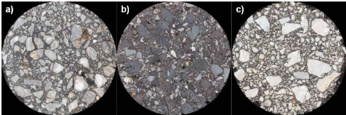
Fig. 7.1 Scanned images of mixtures; (a) AC12.5 surf 50/70 a , (b) AC12.5 surf PmB (SBS) and (c) AC20 base 50/70
