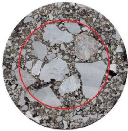
Fig. 7.7 Inner and outer region definition for segregation analysis
