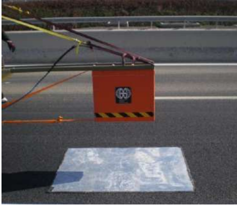
Fig. 4.6 Calibration procedure using a metallic plate
