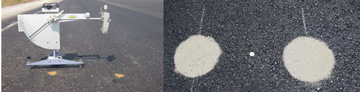
Fig. 9.7 Field microtexture and macrotexture measurements
