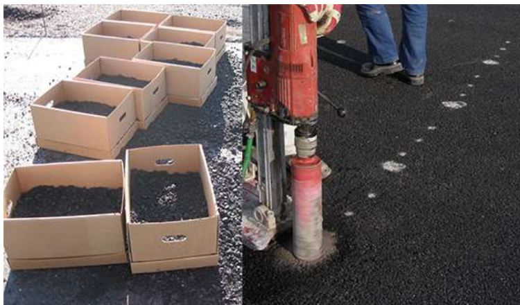
Fig. 3.1 Mix sampling (left) and field coring (right)
