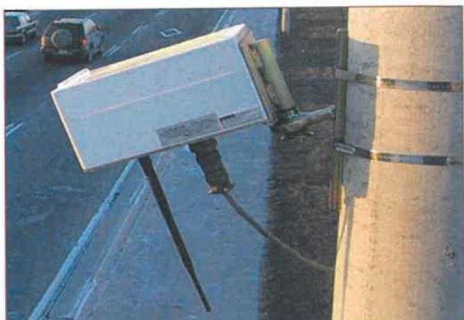
RTMS (Remote Traffic Microwave Sensor) radar
