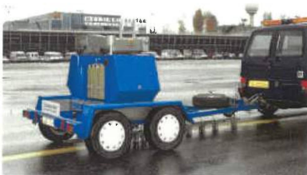
Σχήμα 3.5: Το Falling Weight Deflectometer Dynatest 8002 ( www.dynatest.com/hardware/fwd_hwd.htm )
