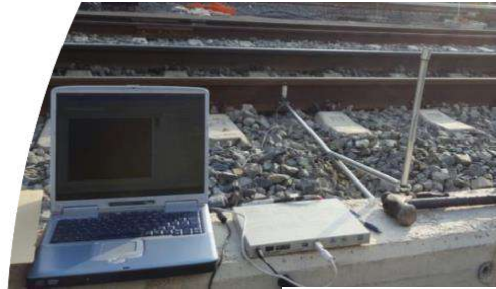
5SM/3G enabled, GPS device based on ATmega328 (Arduino)
